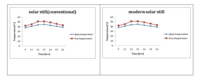
As the modern still is maintaining its temperature for long time it is also producing more yield compared to conventional solar still the yield of both the stills starts from 9:00AM and the increases during 1:00PM and then gradually decreases as the sun sets. The modern still gives up to 1.44L/m2 in comparison to conventional solar still which gives 0.94L/m2 the black ink with 0.3% concentration in water which increases the yield by 34.3% in winters of January 2025 as shown in figure 4:
